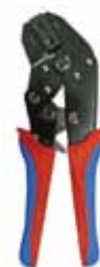
KT32057 PRE-INSULATED FLAG TERMINAL CRIMPER CRIMP RANGE: 20 - 18AWG, 16 - 14AWG 0.5 - 1MM 2 , 1.5 - 2.5MM 2 LENGTH: 230MM WEIGHT: 0.6KG
