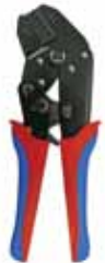
KT32053 BOOTLACE FERRULE CRIMPER CRIMP RANGE: 20AWG - 10AWG 0.5 TO 6MM 2 LENGTH: 230MM WEIGHT: 0.6KG
