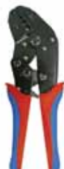
KT32055 COAXIAL CABLE CRIMPER CRIMP RANGE: RG58,59,62,8X,140,141 174,210,223,303,400 1.0 TO 6.5MM 2 LENGTH: 230MM WEIGHT: 0.6KG
